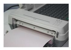
Wide paper design recorder with precise positioning function, supporting Folded /Reel thermosensitive printing paper
