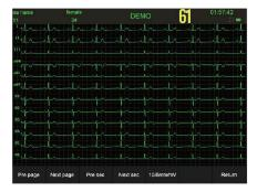
Support saving 300 seconds digital 24 bit uncompressed waveform Random 10-second waveform can be chosen for analysis & processing
