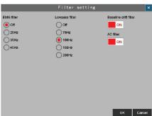
Support four kinds of filter setting: AC filter, baseline drift filter, EMG filter, lowpass filter. High-speed baseline correction filter ensures rapidly correcting the baseline
